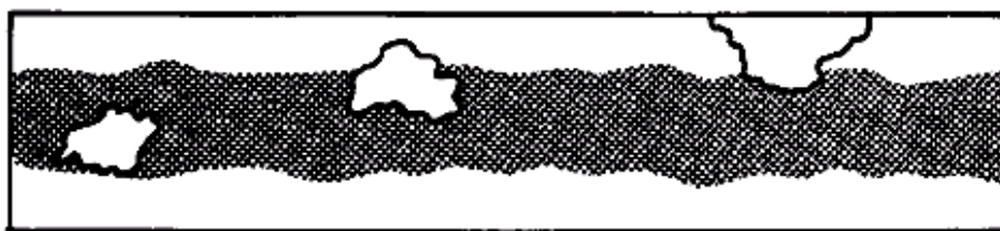
Figure 244-4-13. Chunking Out of Stave Bearing
